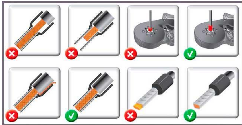
Figure 3 Cable Ferrule Mounting Procedure
