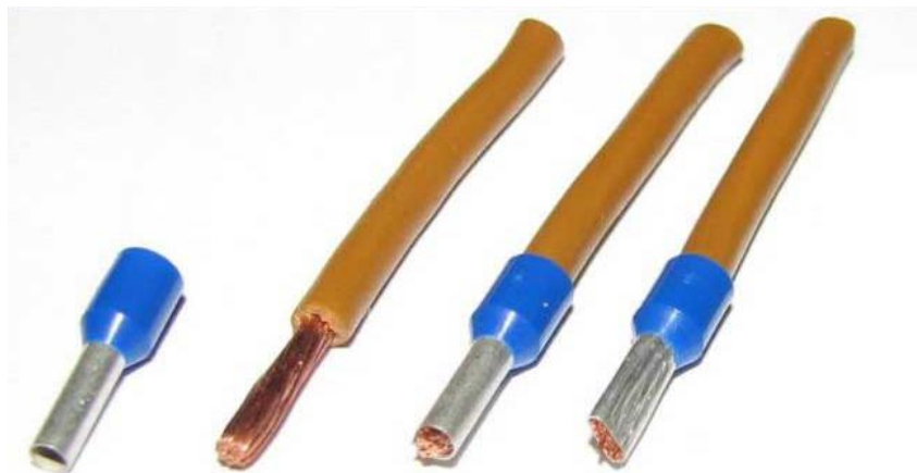
Picture 13 Example of Mounting a Cable Ferrule on the Stripped Core of Multicore Cable
